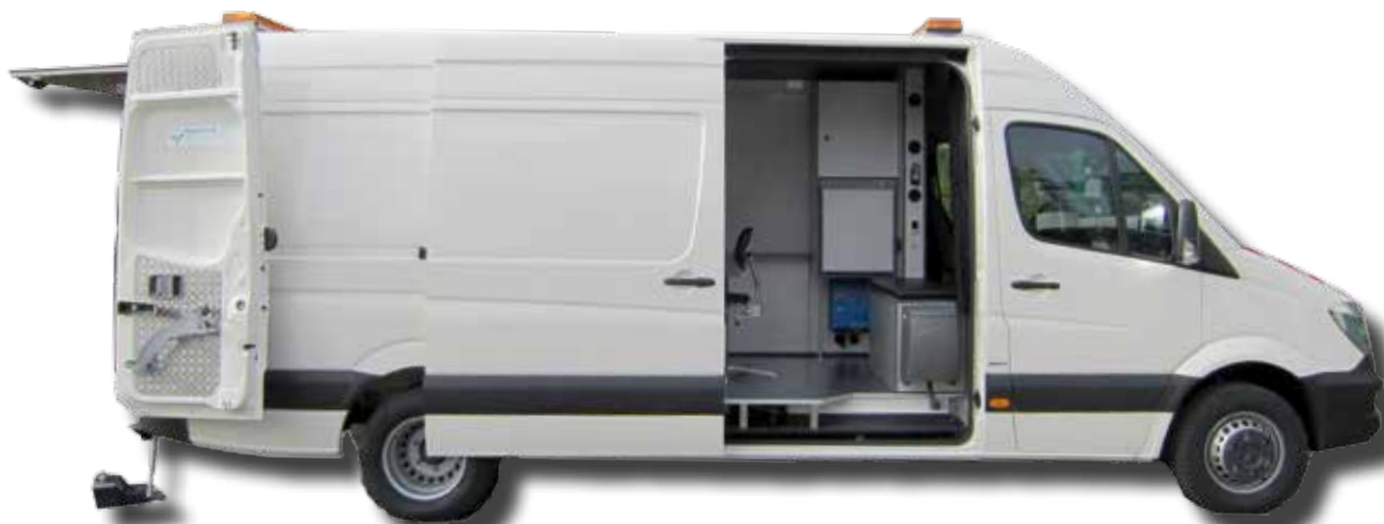
Motor vehicle with the permissible total weight of 5.0 to, with co-driver rotating seat and swing doors 270°
